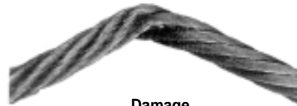
Damage caused by improper use, (e.g. by fixing a load with the rope)
