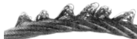
Loop formation on wire rope
