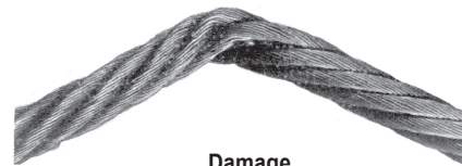
Damage caused by improper use, (e.g. by fixing a load with the rope)
