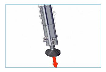
31. To decrease height depress lever and push foot up to desired position.Observe gantry is level.
