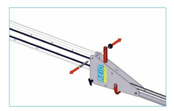
28. Move leg assembly to required position.
