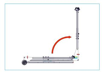
12. Rotate second leg assembly to vertical position and place first leg assembly back down.
