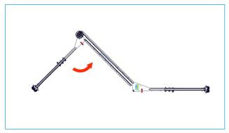
9. Replace pin into hole ensuring the pin is fully engaged through hole.A gentle rocking motion can be used to induce
