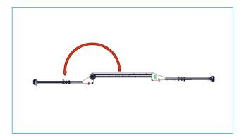
8. Scissor leg assembly until aircraft/ball-lock pin is adjacent to beam.
